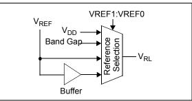
FIGURE 5-3: Resistor Ladder Reference Voltage Selection Block Diagram.
