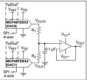
**FIGURE 8-6:** Simple Double-Precision DAC using MCP48FEBX2.
