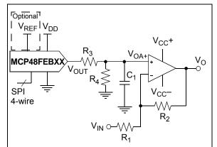
**FIGURE 8-4:** Digitally-Controlled Bipolar Voltage Source Example Circuit.
