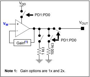
FIGURE 5-5: Output Driver Block Diagram.
