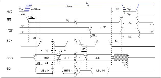
FIGURE 1-5: SPI Timing (Mode = 00) Waveforms.
