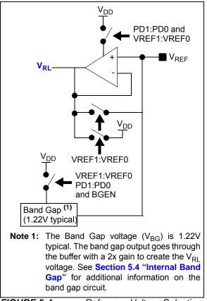
**FIGURE 5-4:** Reference Voltage Selection Implementation Block Diagram.
