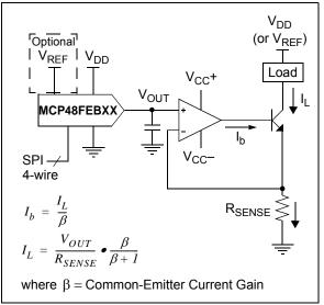
FIGURE 8-7: Digitally-Controlled Current Source.
