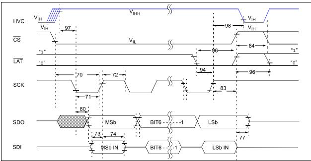
FIGURE 1-4: SPI Timing (Mode = 11) Waveforms.
